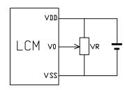
$V_{DD^{\sim}}V_0\text{: LCD Driving voltage}$
